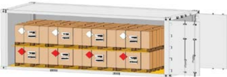
Above: IMDG Placard requirement for two dangerous substances, both with a single hazard class.
